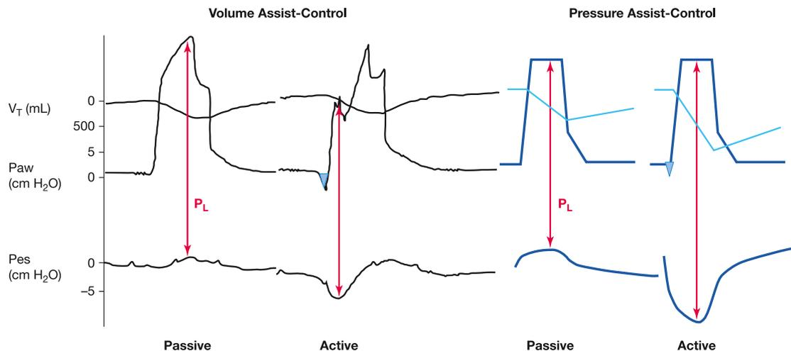
**Figure 2.** Comparison of volume-assist control and pressure-assist control ventilation with recordings of tidal volume ( $V_T$ ) and airway and esophageal pressure ( $P_{aw}$  and  $P_{es}$ , respectively) waveforms. The red arrows illustrate the difference between airway and esophageal pressure, that is, transpulmonary pressure or  $P_L$ .  $P_L$  increases with the patient's effort only during pressure control.
